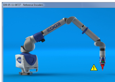
Figure 3-4 Unknown FARO i-Probe warning
