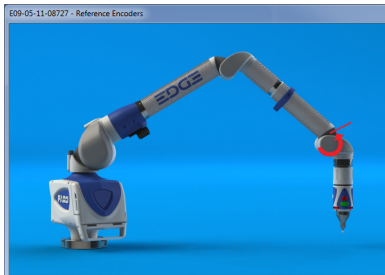
Figure 3-2 Edge end stop warning
